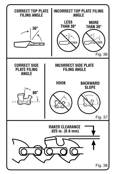
Use a Flat File and a Depth Gauge Jointer to lower all gauges uniformly. Depth gauge jointers are available in .020 in. to .035 in. Use a .025 in. depth gauge jointer. After lowering each depth gauge, restore original shape by rounding the front. Be careful not to damage adjoining drive links with the edge of the file. *See Figures 39 - 40.*
